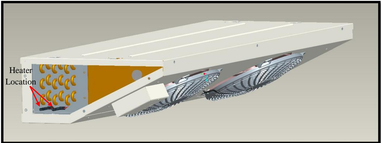
Heater slot available for defrost heaters and it had been inserted into the lower of cooling coil. It is advised to install thermal fuse (supplied by site) when the unit is used with defrost heater. The location of the thermal fuse should be appropriately located to have safety cut off when the heater is overheated.
