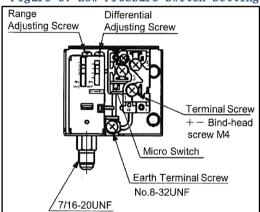
The pressure switch fitted to condensing units with auto reset for low pressure is factory preset to 1.0 bar cut-out. **Do not set low pressure cut-out lower than factory default setting.**
