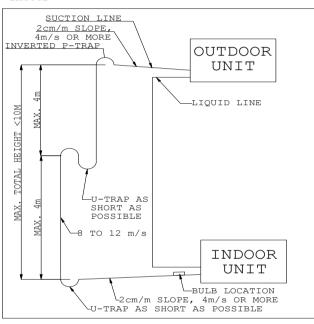
Figure 11: Piping Layout for Outdoor Below Indoor
