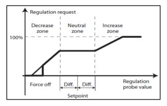
When the suction pressure falls inside the neutral zone (setpoint  $\pm$ - differential), the capacity is stable and there is no loading or unloading of the digital scroll compressor.
