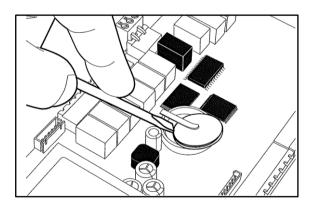
The battery in the controller should be changed every three years.
