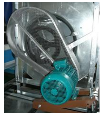
Figure 8: Fan - Motor Assembly
