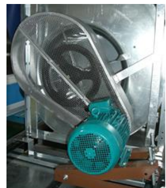
Figure 8: Fan - Motor Assembly
