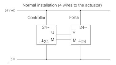
50VA transformer required per actuator.
