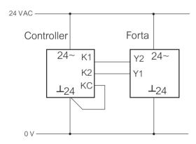
50VA transformer required per actuator.
